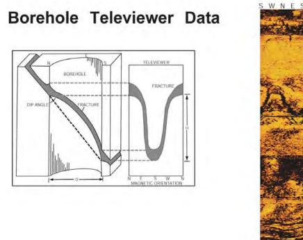
Each identified feature was digitized using WellCad software which then calculates the dip and dip direction of the features taking into account the borehole tilt and orientation.
